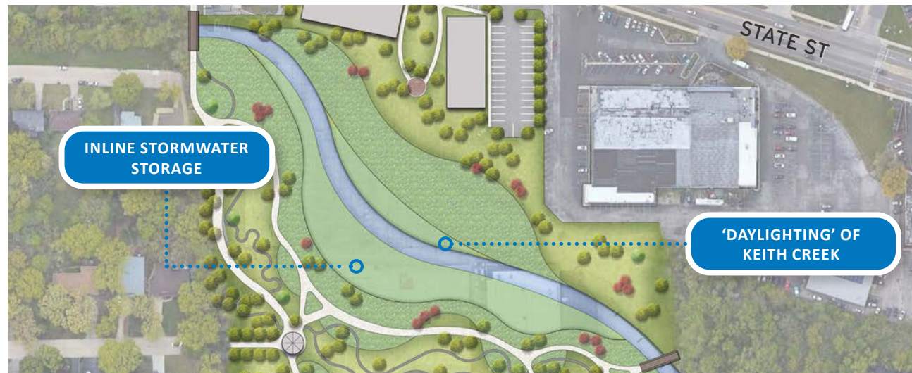
FIGURE 29: ALPINE HILLS AND ALPINE PARK STORMWATER MANAGEMENT
